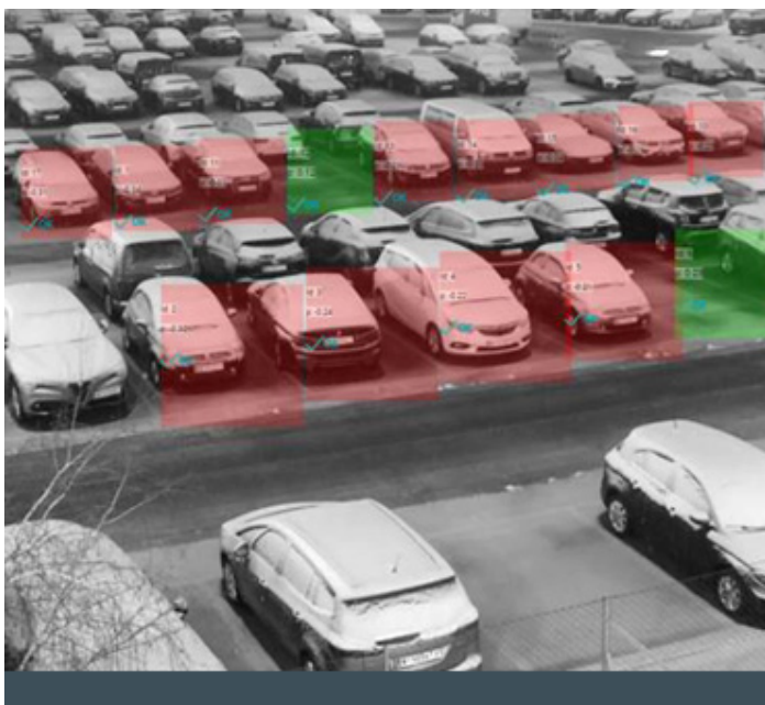
Stationary cameras mounted above a surface lot can detect space availability.
