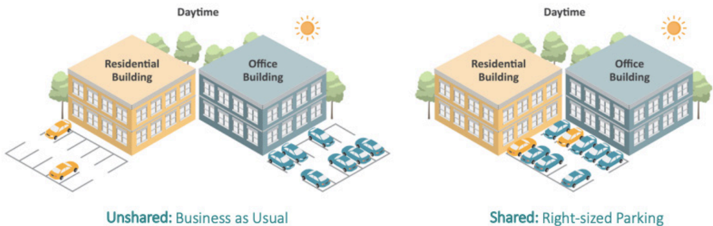
Diagram of shared parking agreement between a residential development (with higher nighttime demand) and an office (with higher daytime demand).
